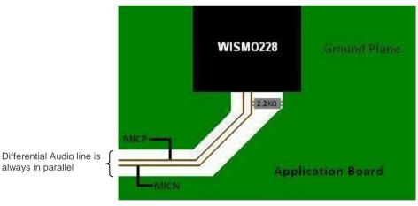
Figure 23. Differential Audio Connection
