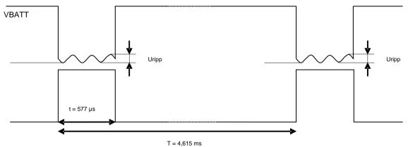
Figure 2. Power Supply During Burst Emission
