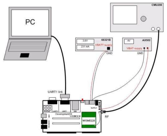
Figure 42. Typical Hardware Configuration
