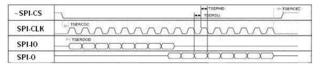
Figure 4. SPI Timing Diagram
