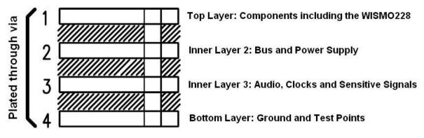
Figure 44. PCB Structure Example for the Application Board
