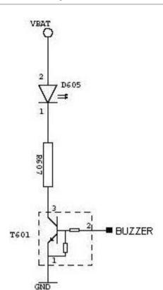
Figure 29. Example of an LED Driven by the BUZZER Output
