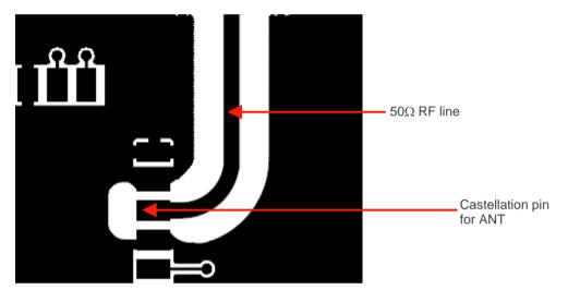
Figure 41. Example of a  $50\Omega$  RF Line
