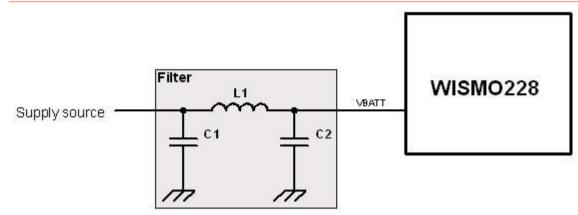
Figure 3. Reject Filter Diagram
