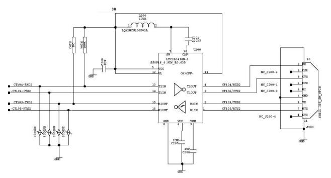
Figure 6. Example of an RS-232 Level Shifter Implementation for UART2
