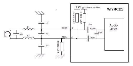
Figure 15. Example of a Differential MIC Connection with an LC Filter
