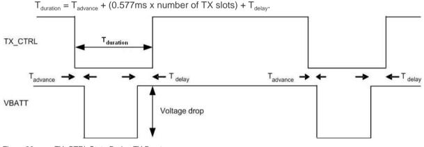
Figure 36. TX\_CTRL State During TX Burst
