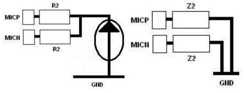
Figure 13. DC and AC Equivalent Circuits of MIC
