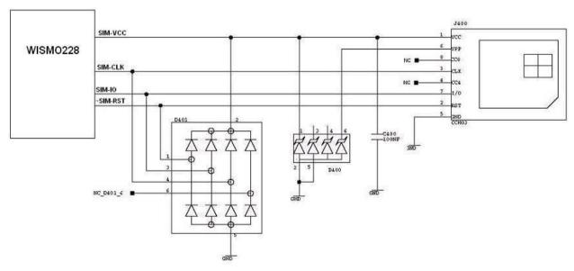
Figure 12. Example of a SIM Socket Implementation
