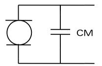
Figure 21. Capacitor Soldered in Parallel to the Microphone
