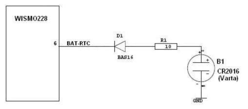
Figure 34. RTC Supplied by a Non Rechargeable Battery
