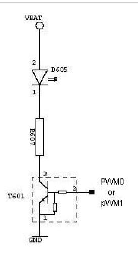
Figure 26. Example of an LED Driven by the PWM0 or PWM1 Output
